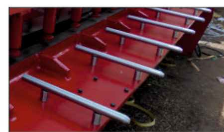
Sandwich type bolted i-box design for mounting of holding cylinder to facilities the maintenance
